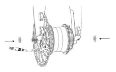
4. Fasten clockwise BC3/8 cap lock-nuts with open-end wrench at both ends of the motor. Torque requirement: 30-36N.m.
